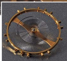
Screwed balance wheel with hairspring
