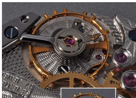
Screwed balance wheel with hairspring
