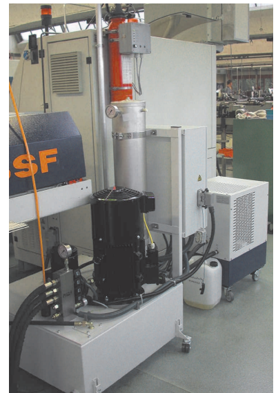
350 bar high pressure pump with cooling unit, oil mist suction and extinction device.
