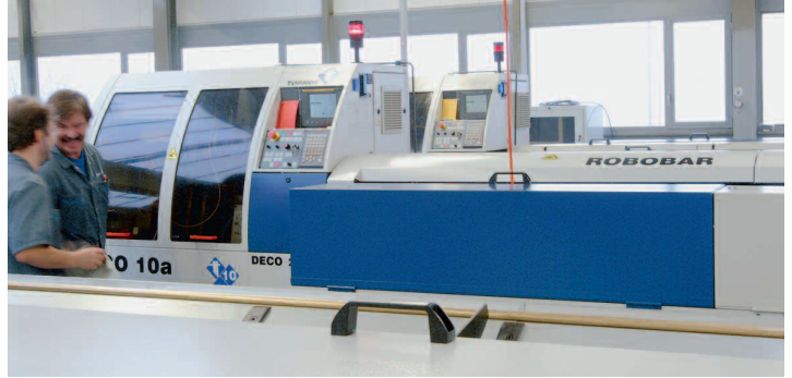
In 2005, we purchased 3 new single spindle PNC-machines of the type Tornos DECO 2000/10.
