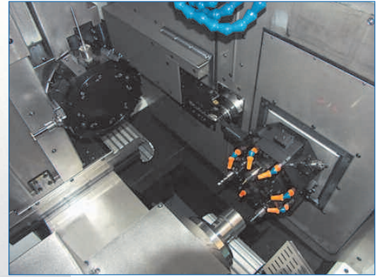
A peek into the machine room with the two tool revolvers with 16 tools each.
