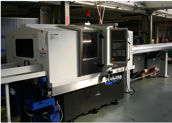
The new Maier machine with 15 spindles and high pressure pump
